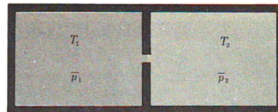
Fig. 7·12·4 A container divided into two parts by a partition containing a small hole. The gas in the two parts is at different temperatures and pressures.
